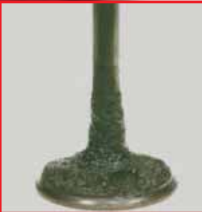
Intake valve before P.i. treatment
