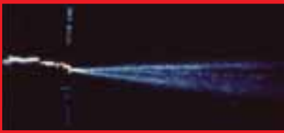
Injector spray pattern before P.i. treatment
