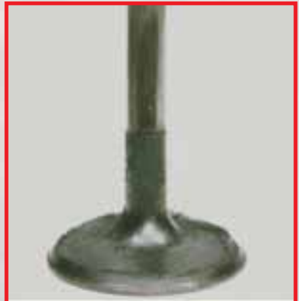
Intake valve after P.i. treatment
