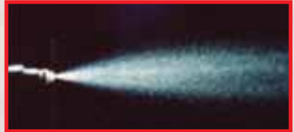
Injector spray pattern after P.i. treatment
